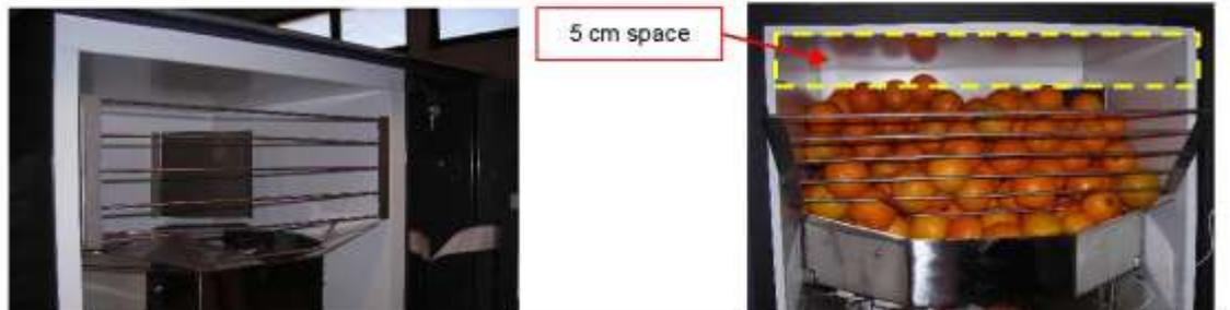
Always leave 5 cm of space in the upper part of the feeding bin to allow the stored oranges to rotate without pushing against each other.
