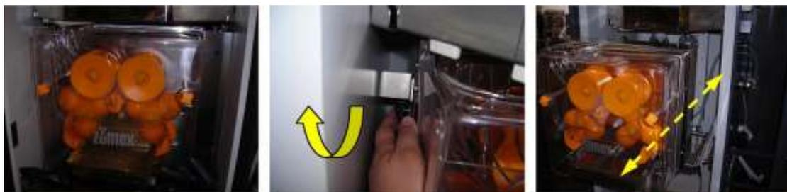
To easily move the pressing unit to the outside, it is necessary to remove the silicon tube from the juice tray.
