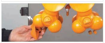
5. Pull off the peel ejectors.
